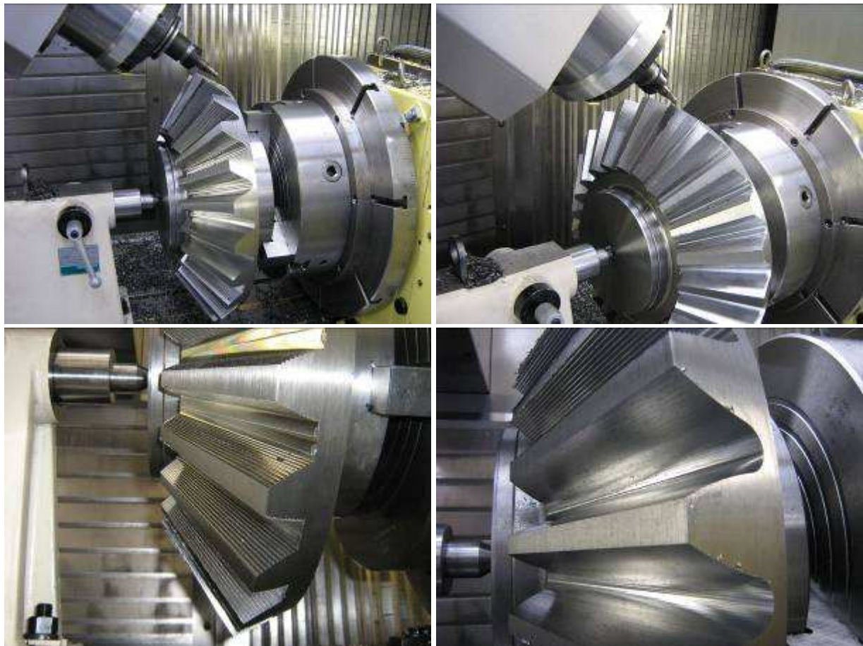
fig. 9 : different steps of bevel pinion milling
