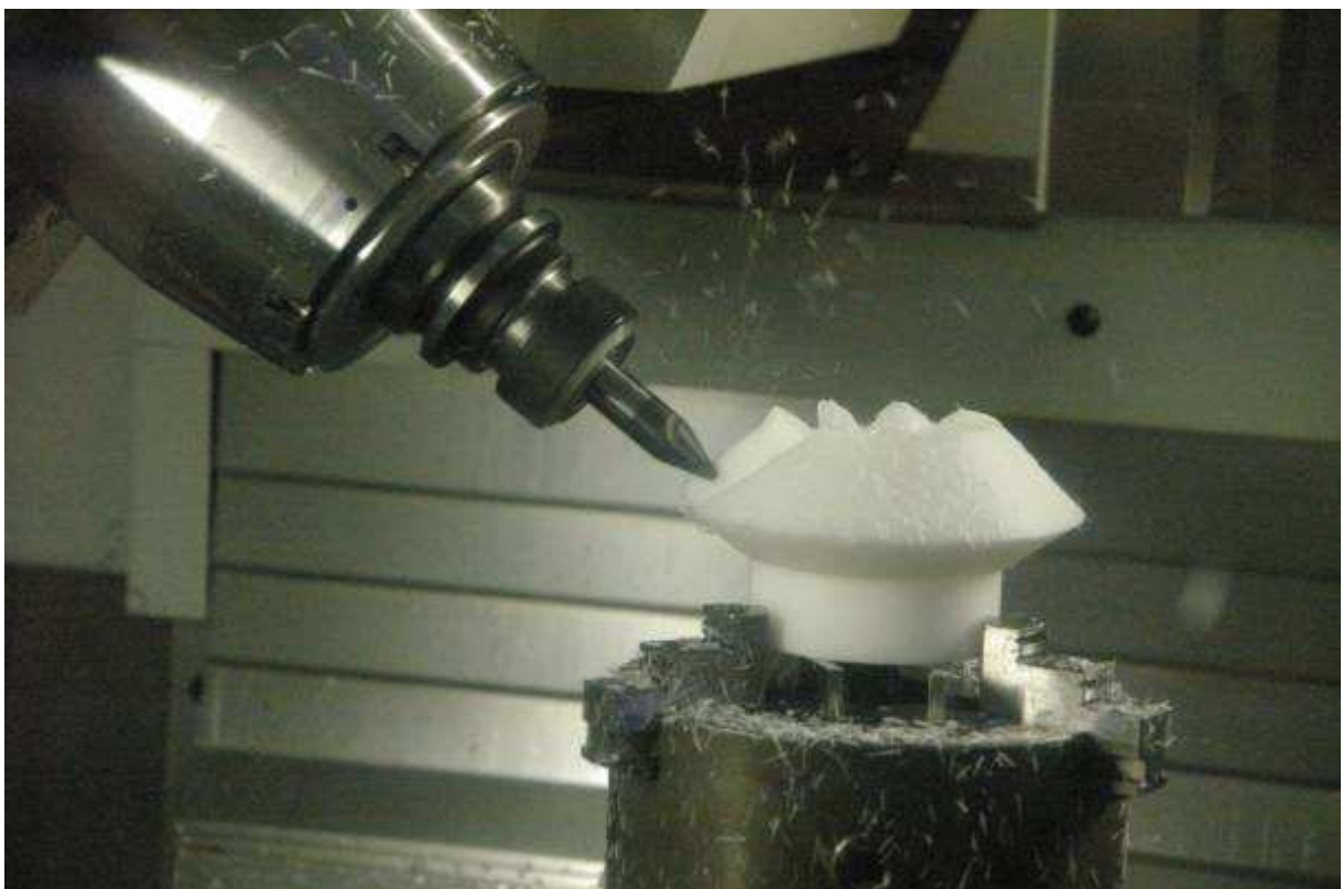
fig. 7 : plastic spiral pinion milling
